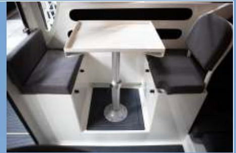
PORT DROP DOWN TABLE SEATING WITH TOP ENTRY STORAGE AND REMOVABLE BACKREST
