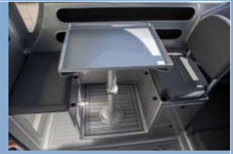
PORT DROP DOWN TABLE SEATING WITH TWO DRAWERS AND TOP ENTRY STORAGE WITH REMOVABLE BACKREST
