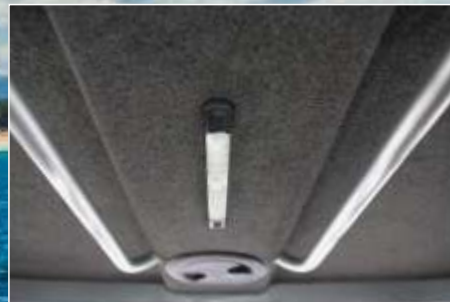
INTERNAL LIGHTING KIT (STRIP LIGHT IN FWD CABIN AND INNER HARD TOP)
